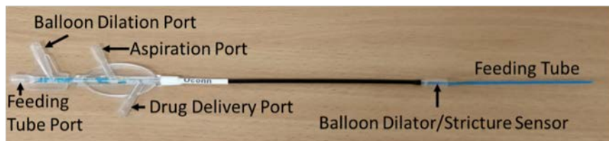
Figure 1. Complete 4-in-1 esophageal tube. This device would be placed in a neonatal patient using radiographic guidance and would allow for immediate feeding following repair of esophageal atresia, as well as fluid sampling, drug delivery, and serial dilations- all without requiring additional anesthesia.
